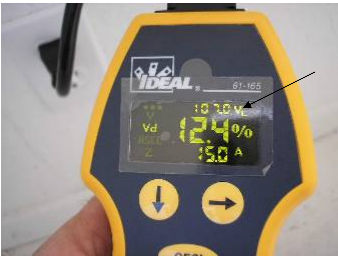
Many of the receptacle outlets had excessive voltage drops at the throughout the house. 2002(NEC) 210.19 Conductors
